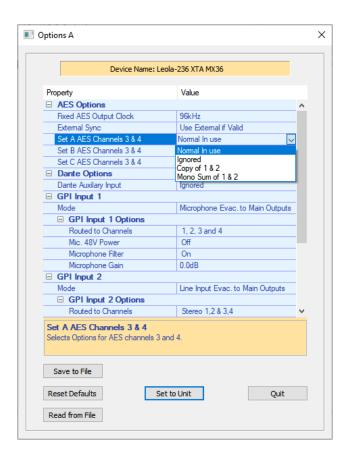
Ignoring channels 3&4 on a set allows the redundancy failover operation to only monitor for a valid AES signal on a set's 1&2 inputs, useful in situations when the console only provides a single AES copy of the main L/R outputs.
