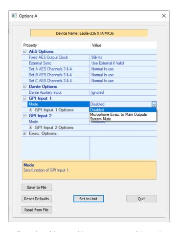
GPI Input 1 can be configured to either provide a system mute of the main outputs, or to route the mic input to selected outputs.
