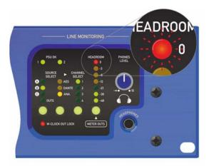
The attack time on this monitoring is instantaneous, but it has a 3 second hold time so even the shortest peaks will be caught and displayed. To determine which channel (or channels) have hit the threshold, cycle through all connected channels until the meter shows full scale flashing in time with the red LED. In this example it's analogue channel 4 on set A.
