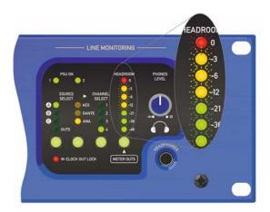
Remember, this is not showing that the unit is clipping – it's an alert to turn down any incoming source level that is close to clipping. The MX36 has output limiters to prevent it from generating a clipped output no matter how many sources are selected.
