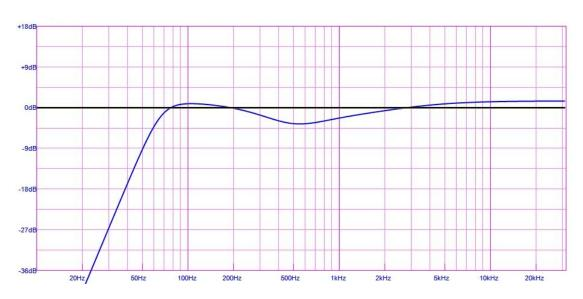
Microphone Input: 24dB/Oct. Butterworth HPF @ 66.2Hz; 500Hz PEQ -3.3dB, Q = 0.84; 1kHz PEQ 2.2dB, Q = 0.4; Channel gain +1.5dB
